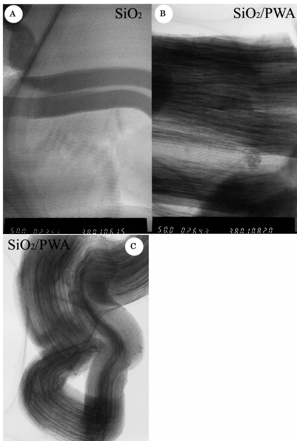
Figure 7 TEM image of mesoporous \text{SiO}_2 (A) and PWA containing mesoporous \text{SiO}_2 (B, C). One can clearly recognize the difference between mesoporous \text{SiO}_2 with and without PWA.
